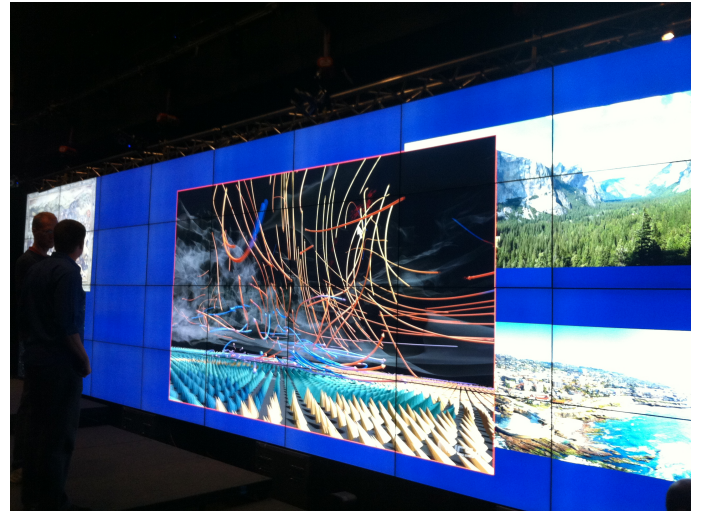
Fig. 3. A 4K video of a tornado simulation rendered in a MediaCommons application via the tiled video playback library [13].
