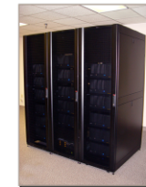
Visualization Cluster: 34 Opteron™ processors with high-end graphics cards, Gigabyte Ethernet, 50 terabyte parallel file system.
