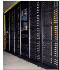
BES System: 284 Opteron™ processors, InfiniBand, 15 terabytes NFS disk storage.
